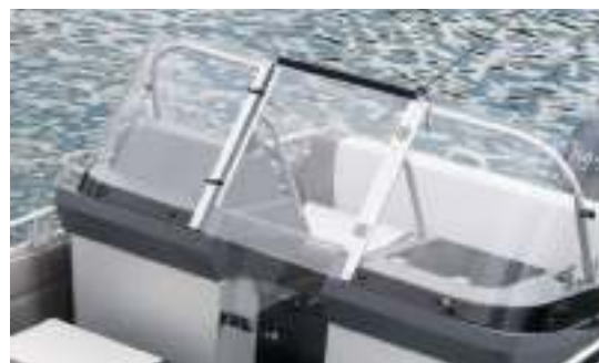
The fixed door between the consoles gives protection from wind and spray
