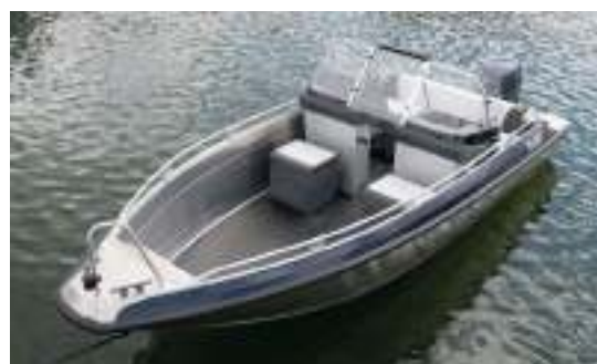
Flexible general arrangement due to the removable seat/stowage boxes
